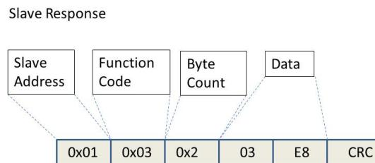
After receiving response from the power meter, Modbus Master acquires the value of currents from the primary-side current transformer (register address 0x000E), which is 1000.
