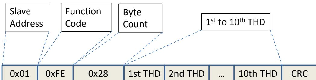
**Note:** The total data length of address 0x702, 0x705, 0x708, 0x70B, 0x70E and 0x711 is 44 bytes.
