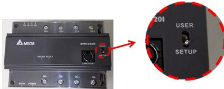
2. Set the communication parameters: Station1, RTU communication mode, baud rate 9600 bps, 8-bit data length, NONE for Parity and 1 for stop bit.
