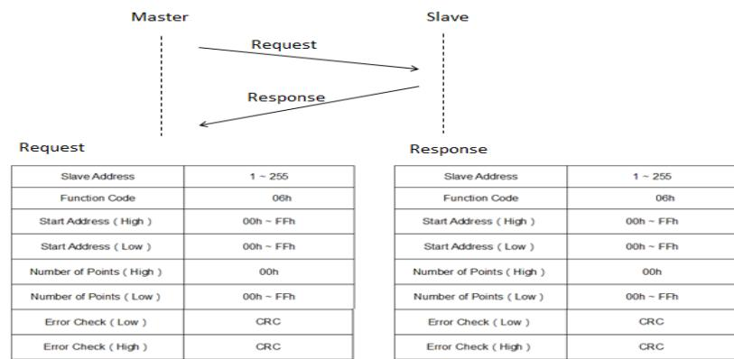
Example: If Modbus Master such as PLCs or data collectors reads values of CT's primary current (Register address 0x000E) of the power meter (Modbus Slave)(Slave address is 0x1) by using Modbus protocol, which the register value would be 1000.
