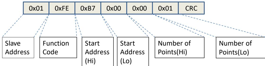
The following is packet format of Response sent by Modbus Slave (The part before Byte Count is same as Modbus RTU.)
