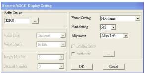
Click [...]. In the **Refer Device** dialog box, choose the VFD communication port that you need. If you want to read the output frequency (H), set the **Absolute Addr.** to 2202. For other values, refer to the ACMD Modbus Comm Address List.
